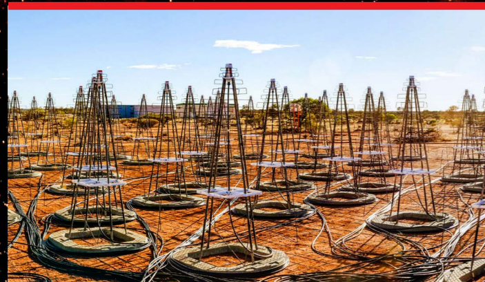
Right: Part of the AAVS Test Platform comprising of "Christmas Tree" antennas at the Murchison Radio-astronomy Observatory in outback Western Australia.
